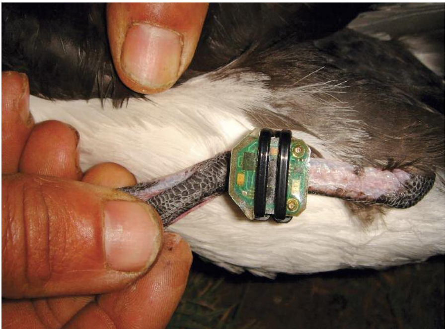
Figure 1. A 2.5g British Antarctic Survey Geolocator attached to a Manx Shearwater's leg. The geolocator records daily positions and flight activity throughout the annual migration.
