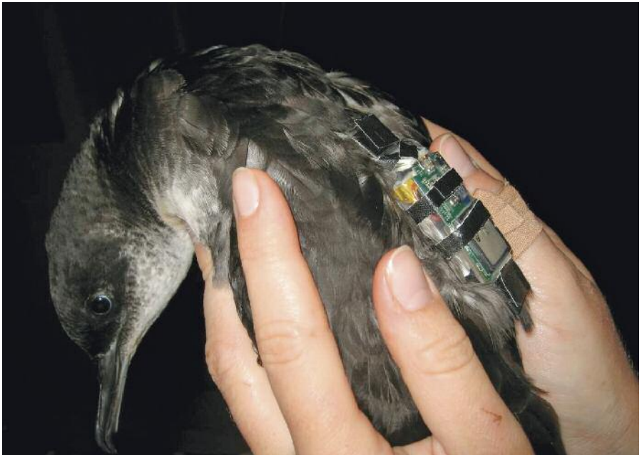
Figure 2. A 15g GPS logging device attached to a Manx Shearwater's back feathers using marine tape. The device records accurate positions every five minutes to reveal the bird's foraging movements.
